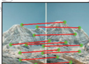
Purifying algorithm for rough matched pairs using Hough transform (P1017)
